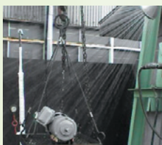
(Reference) IP44 spray test Rotating machine protected against splashes
